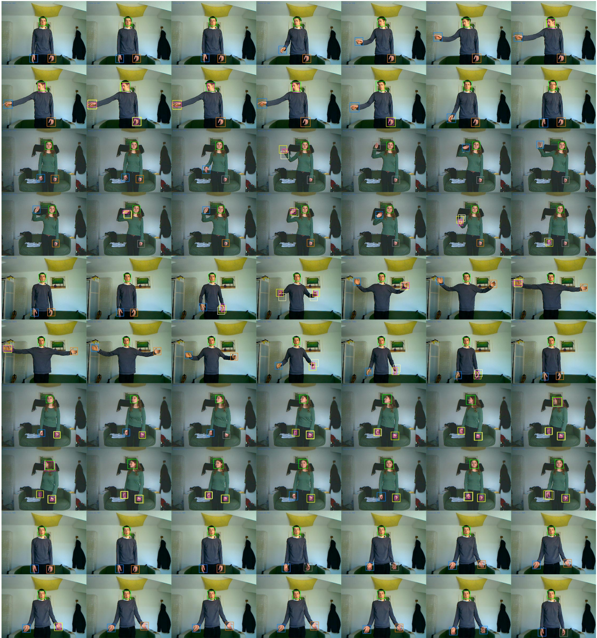
Fig. 7.10: Gestures used for our final experiment with drawn in detection results. The first two rows show the pointing gesture. The second two rows the waving gesture. The middle two rows depict the thisbig gesture. The second last two rows show arbitrary movements with the arm, i.e., a non-gesture. The last two rows illustrate the dunno gesture.
