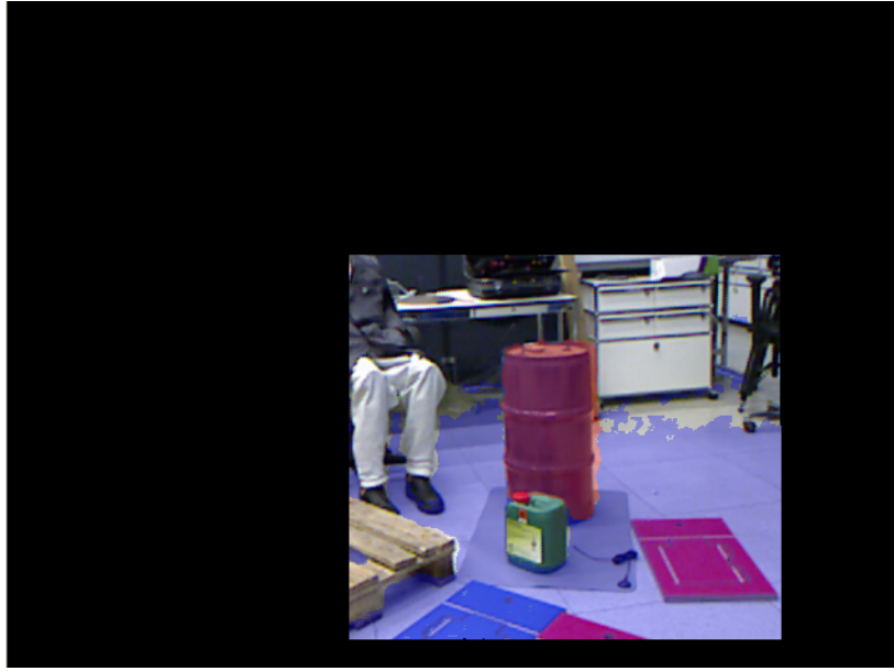
Figure 4.8: Assigning the whole parts of the object as foreground, for all pixels which have the similar depth values as the seed pixel.
