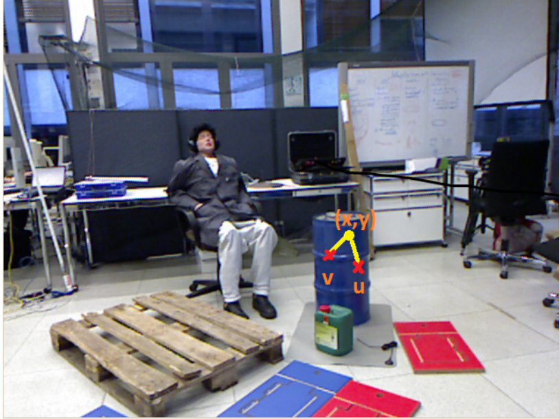
Figure 4.13: In this Figure, the two offsets u and v are both on the object, and the depth difference or color difference between them is not big.
