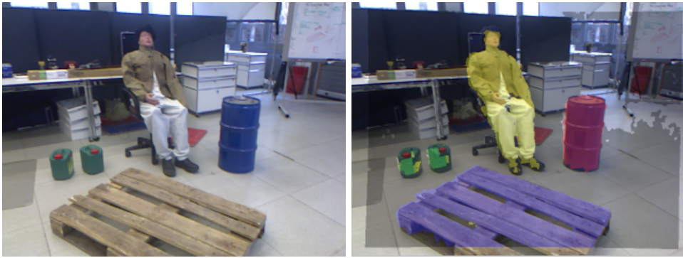
Figure 3.10: Object-class segmentation. The image on the left is the input image. Right image is the object class segmented image. The objects of interest are human labelled with yellow, canister with green, pallet with blue, and barrel with red.
