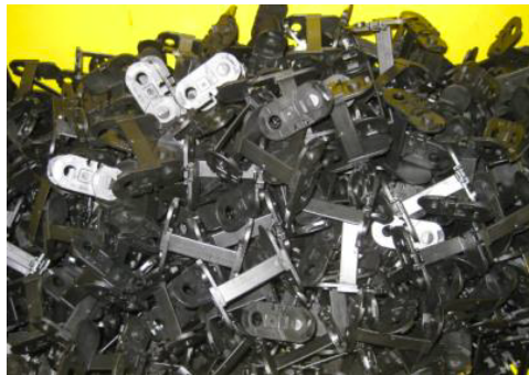
Figure 3.1: The bin with parts lying in a random pile when supplied after production.
