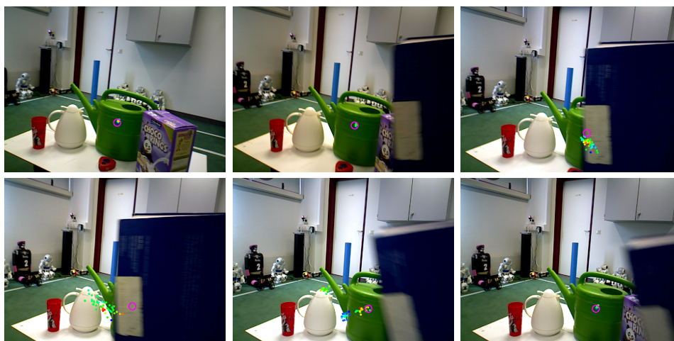
Figure 4.15: Reinitialization: While tracking (top left), the target is covered with a book (top centre). Tracking is maintained with over 50% occlusion (top right). Bottom left: The track is lost with the object almost totally occluded, and reinitialization occurs (bottom centre). Bottom right: the track is recovered from the new hypotheses. [The ground truth is shown as a pink circle, while the particles are shown as dots coloured according to weight (red for high, blue for low)]
