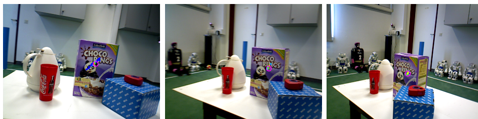
Figure 4.17: Orientation uncertainty: With only one side of the box visible to the camera, the uncertainty in camera orientation grows (left), when more of the object comes into view, the estimate improves (centre). The estimate remains good despite partial occlusion of the object (right).
