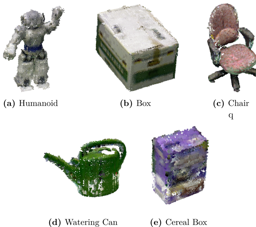
Figure 4.2: Learned Object Models visualized by samples from the surfels at 2.5cm resolution.
