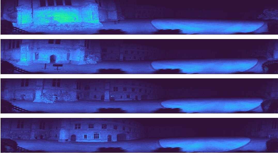
Figure 2.4: Multiple 2d projections taken from the Newer College Quad-Easy dataset. Images are colored by the recorded intensity value clamped to range [0, 0.35 \cdot I_{max}] . The scans are taken 40 LiDAR frames apart. The image center is the forward direction for sensor movement.
