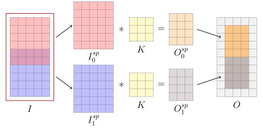
(b) The split edges in the output are restored by computing the area along the edge twice. Once in  $I_0^{sp}$  and once in  $I_1^{sp}$ . The outer border cannot be computed without padding I.
