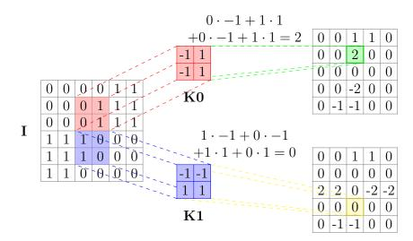
**Figure 3.1:** Convolution operation applying two 2D kernel K0, K1 onto a 2D input I
