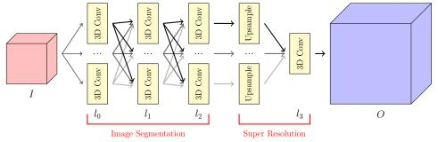
(c) The smallest super resolution network tested is a 4 convolutional layer network. It consists of a 3 layer image segmentation stage with the 3 multi channel convolutional layers  $l_0$ ,  $l_1$  and  $l_2$  followed by a multichannel upsampling layer and a single channel convolutional output layer  $l_3$ .
