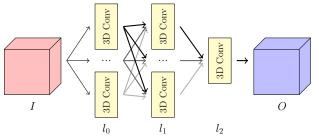
(b) The 3-layer image segmentation network has two multichannel convolutional layers  $l_0$  and  $l_1$  and one single channel output layer  $l_2$ .
