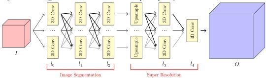
(d) The 5 layer super resolution network consists of the same image segmentation stage as the 4 layer variant. The super resolution stage consists of the upsampling layer followed by a multichannel convolutional layer  $l_3$  and a single channel convolutional layer  $l_4$  generating the output O.
