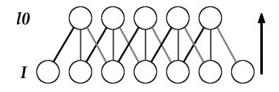
Figure 3.3: Applying the convolutional layer l0 with kernel size 3 onto input I with  $size_{inp} = 7$  reduces the  $size_{out}$  to 5
