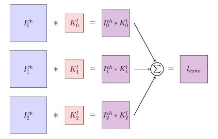
**Figure 3.4:** Applying a convolutional layer l with  $ch_{in} = 3$  input channels and  $ch_{out} = 1$  output channels onto an input I with channels  $I_0^{ch}$ ,  $I_1^{ch}$  and  $I_2^{ch}$ . The parameters of the convolutional layer are the convolution kernels  $K_0^l$ ,  $K_1^l$  and  $K_2^l$ .
