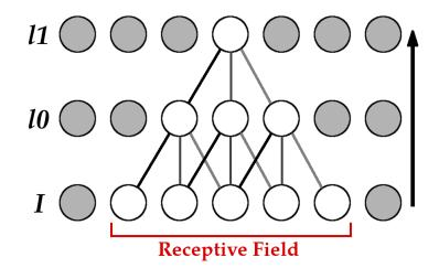
Figure 3.2: 1D Receptive field growing through 2 convolutional layers l0, l1 with kernel size 3, applied onto a 1D input I
