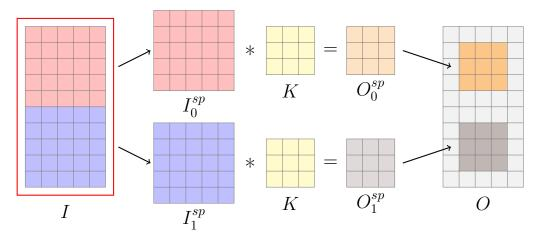
(a) An input I with size 5x10x1 is split into two 5x5x1 subvolumes  $I_0^{sp}$  and  $I_1^{sp}$ . These subvolumes are convolved with kernel K with  $size_K = 3$ . This results in two 3x3 outputs  $O_0^{sp}$  and  $O_1^{sp}$  which when set back together leave a 2x3 gap between the subvolumes. The grayed areas in O are the missing voxels.
