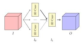
(a) The smallest image segmentation network tested is a 2 convolutional layer network with one multichannel convolutional layer  $l_0$  and one single channel output layer  $l_1$ .
