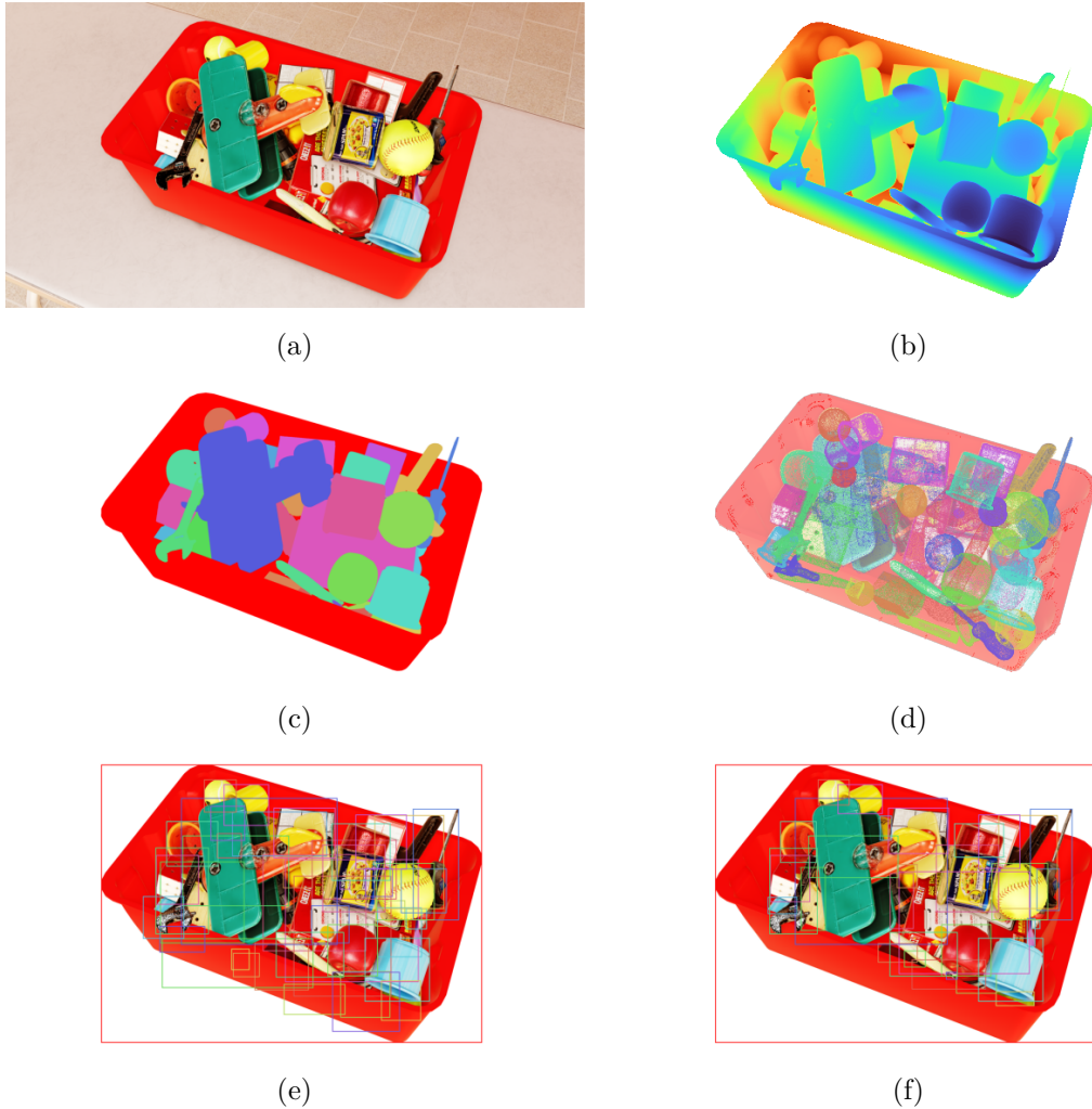
Figure 4.1: Examples from an annotated simulated scene created by our cluttered bin generator. (a): RGB, (b): depth, (c): semantic segmentation, (d): object poses, (e): bounding boxes and (f): bounding boxes shrunk to object visibility.
