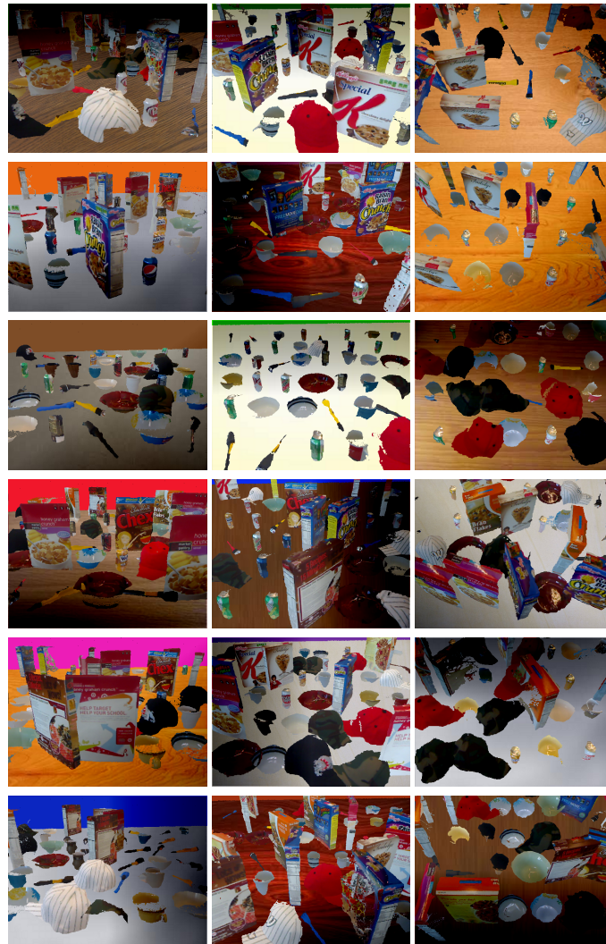
FIGURE 5.4: Negative training images are generated by populating rendered table plane with negative object class.
