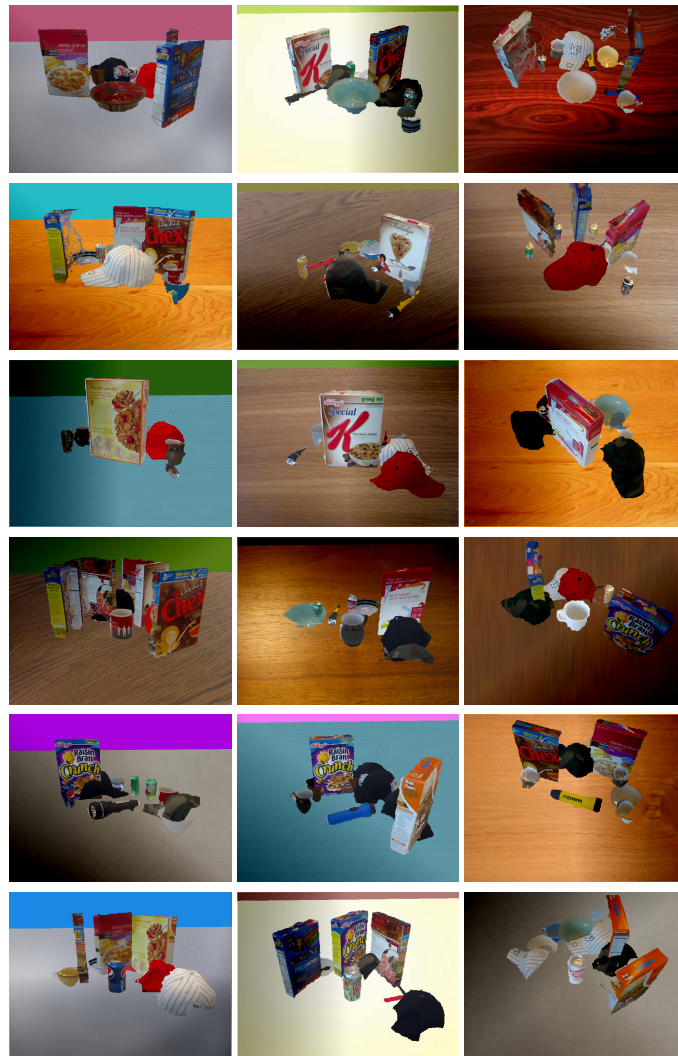
FIGURE 5.3: Positive training images are obtained by placing positive object class instances at the same place and orientation as in RGB-D Object dataset, in order to take advantage of annotations. To simulate clutter and occlusion, object class instance of other classes are placed around the object.
