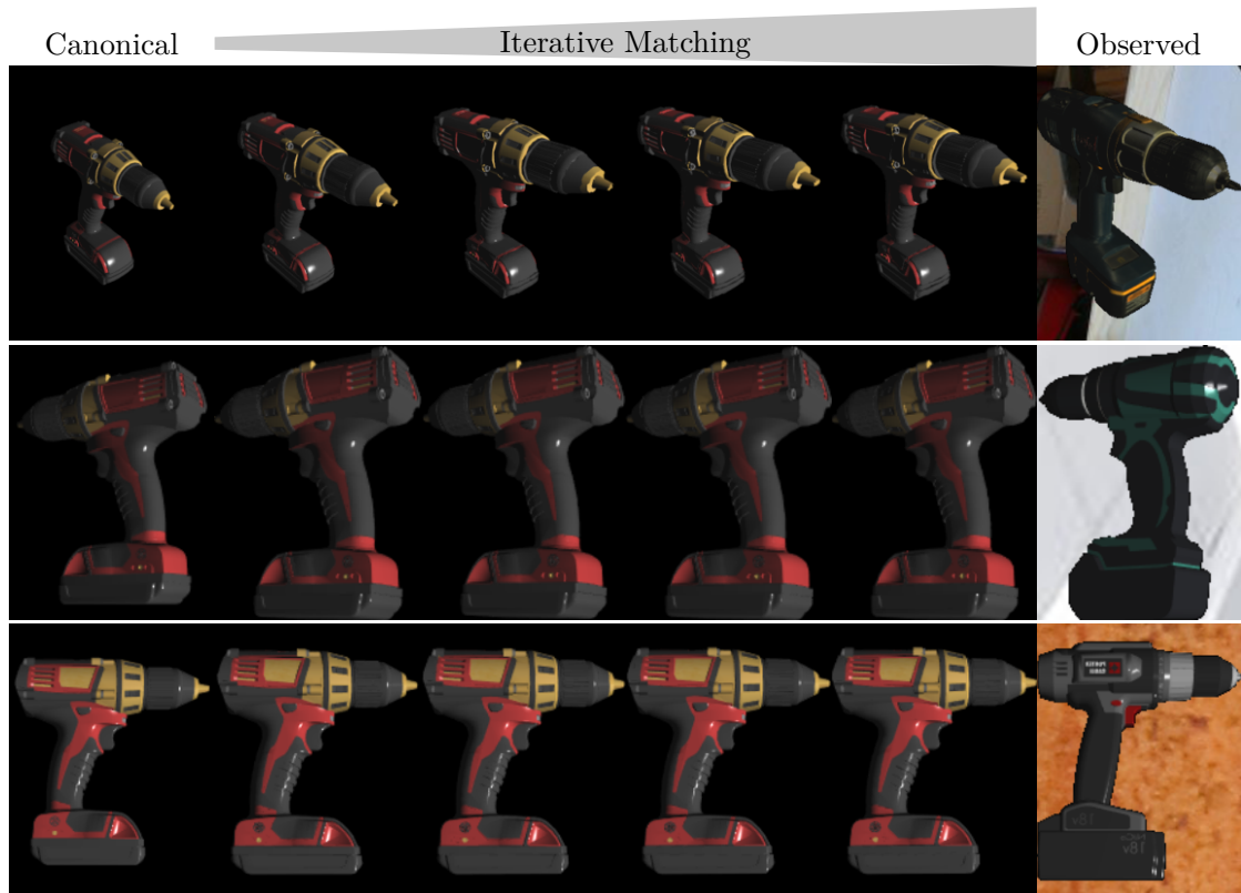
Figure 5.6: Stepwise evolution from the unmorphed canonical model on the left to match the observed model on the right. The examples are chosen randomly and five iterations were made.
