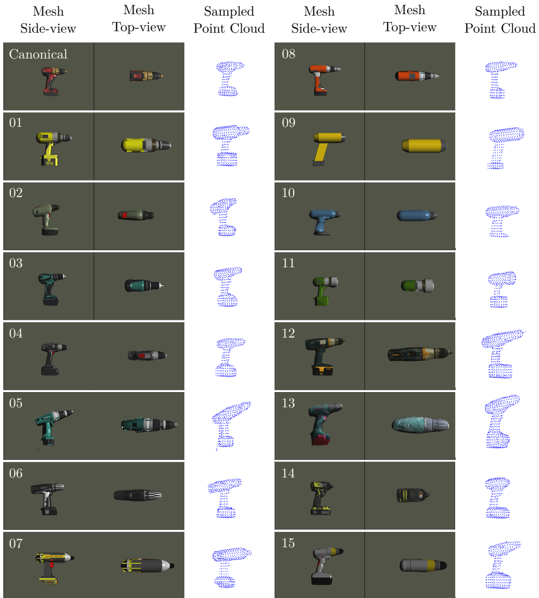
Figure 5.2: Two rendered images from a side and a top view, followed by a visualization of the underlying point cloud for all meshes used to produce the synthetic dataset.
