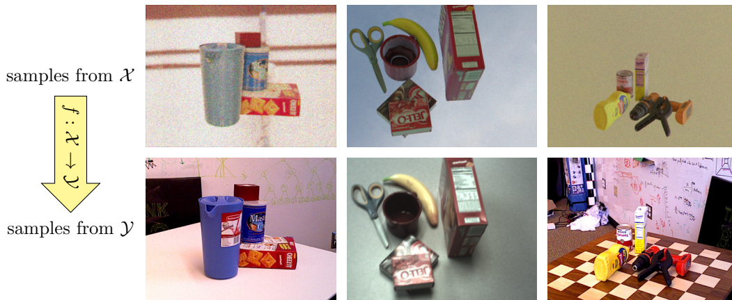
Figure 4.1: Real YCB-Video frames (bottom) alongside corresponding synthetic images (top). It can be seen that, besides the backgrounds, there are visual differences in the object appearance that form the domain gap.
