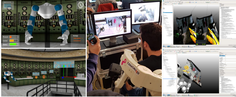
Figure 17: Overview of visualization possibilities: t.l.: head-up display visualization of internal parameters, b.l.: projection of semantic object information via billboard visualizations, c.: first person operator using the exoskeleton with direct camera view and point cloud visualizations, t.r.: stereoscopic and b.r.: third person view on the scene during a manipulation task.
