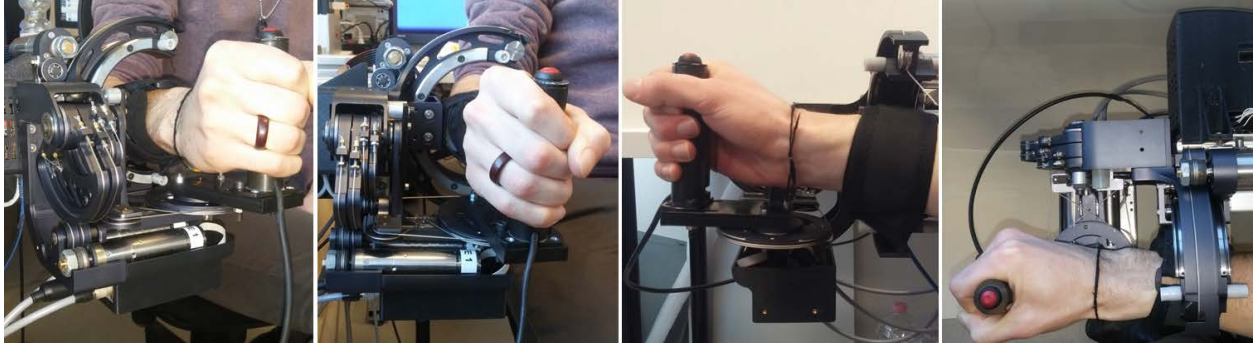
Figure 10: The wrist exoskeleton worn by an operator. Left: Isolated test. Right: Mounted on the arm exoskeleton.
