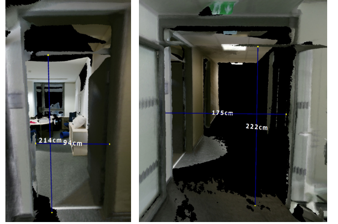
Fig. 9. Examples of interactively taken measurements of heights and widths of a corridor as well as door widths taken to guide the further management process. The real sizes of the doors (i.e. the ground truth values) are 95 cm \times 215 cm (left) and 174 cm \times 222 cm (right).
