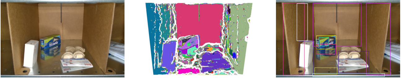
Figure 3. RGB-D based additional region proposals. Left: RGB frame. Center: Regions labeled using the connected components algorithm. Right: Extracted bounding box proposals.
