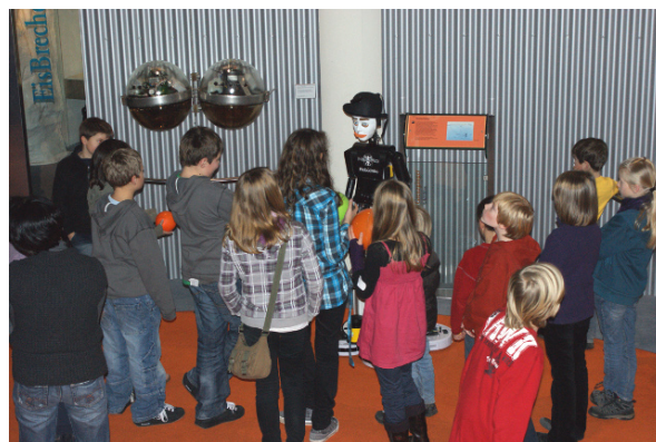
Fig. 1. Our museum tour guide robot Robotinho explains an exhibit at the Deutsches Museum Bonn to a group of children. Visitors listening to explanations usually block the robot's path to its next destination. Clearly articulating the desired motion direction is essential for successful navigation.
