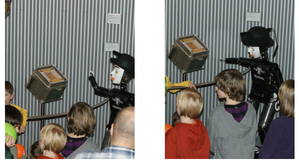
Fig. 4. Robotinho directs the audience's attention to distinctive parts of an exhibit using pointing gestures.
