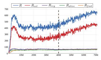
Fig. 4. Training return curves. The vertical dashed line represents the point where the limits of the velocity scheduler have been reached. Note how the agent continues refining the policy after these limits have been reached.
