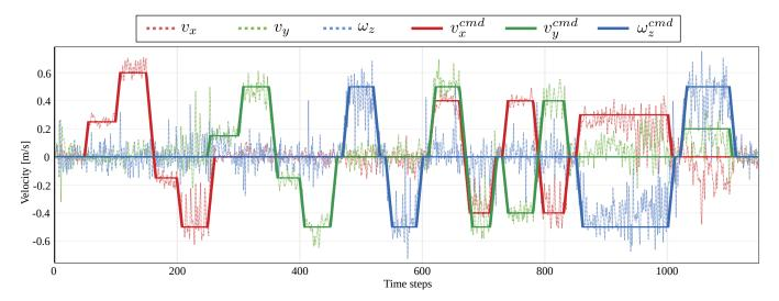
Fig. 3. Velocity tracking. The learned control policy is able to follow the commanded velocities (solid wider lines) in different directions with varying velocities. Initially, motions in single directions (sagittal, lateral and turning) are demonstrated. After 600 time steps, motions with combined directions (sagittal with lateral, sagittal with turning and lateral with turning) are evaluated.
