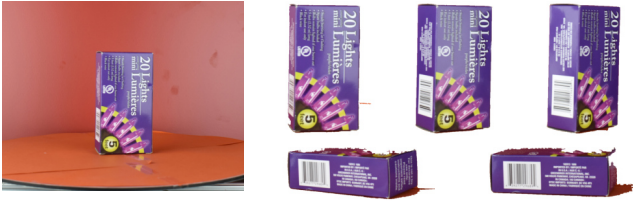
Fig. 5. Turntable capture and automatic segmentation. Left: Input image. Right: Extracted segments in standing and lying configuration.
