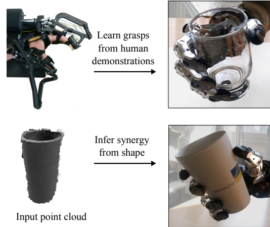
Fig. 1. Grasping configurations of objects in a category are inferred from a description of their shape. Grasping knowledge is encoded in a synergy space and a grasping learner through human demonstrations using an exoskeleton.
