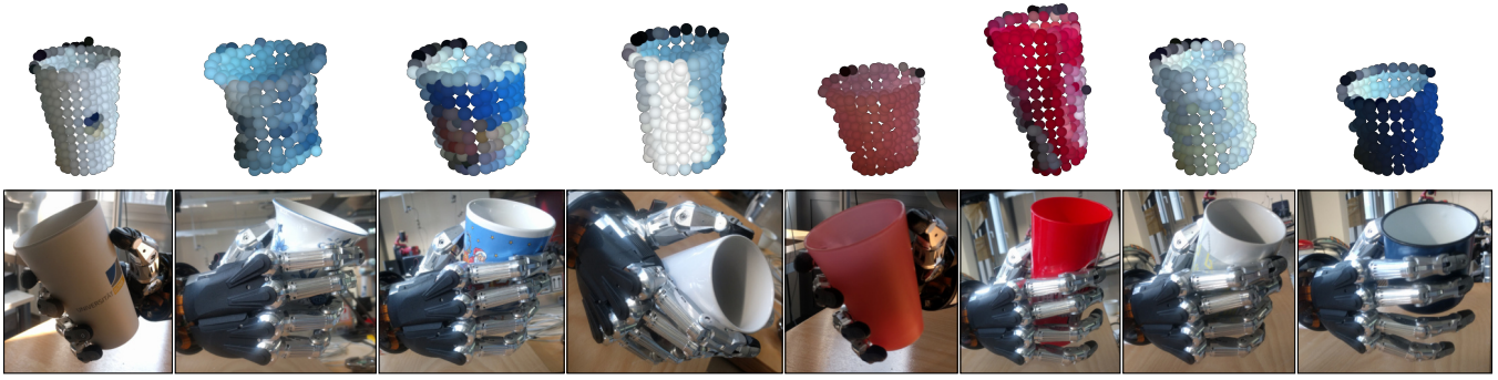
Fig. 12. Real robot experiments for the Glass category. All the objects were presented for the first time to the system and they were successfully grasped.
