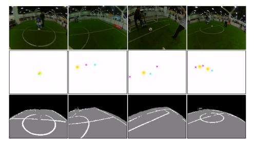
**Fig. 3.** Object detection results. Upper row: captured images by our robots. Middle row: the output of the network with balls (cyan), goal posts (magenta), and robots (yellow). Bottom row: the output of the segmentation branch with lines (white), field (gray), and background (black).
