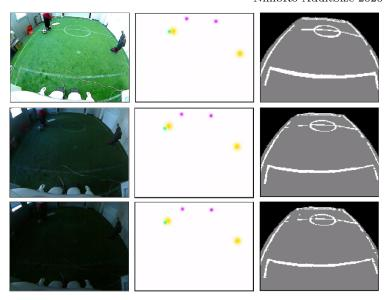
Fig. 4. Object detection under various lighting conditions. Left column: captured images by our robots. Middle column: output of the network indicating balls (cyan), goal posts (magenta), and robots (yellow). Right column: output of the segmentation branch showing lines (white), field (gray), and background (black).
