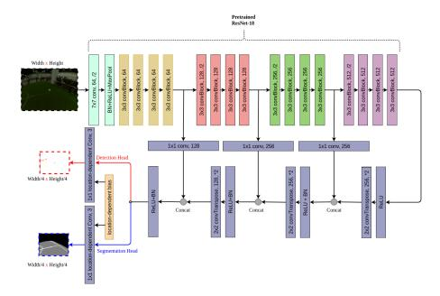
**Fig. 2.** NimbRoNet2 architecture. Similar to ResNet, each convBlock consists of two convolutional layers followed by batch-norm and ReLU activations. For simplicity, residual connections in ResNet are not depicted. Note that instead of a convolutional layer we used a location-dependent convolution in the last layer.
