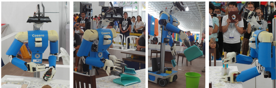
Fig. 6. Tool use demonstrations at RoboCup 2014: Opening a bottle, using a brush and a dust pan, making Caipirinha [17].
