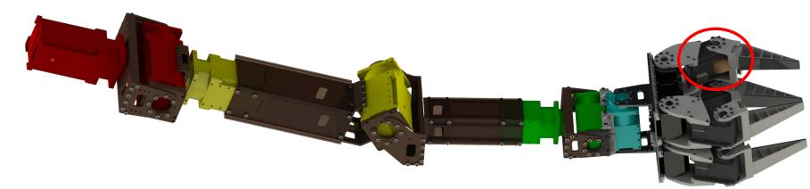
Four fingers with two Dynamixel actuators
